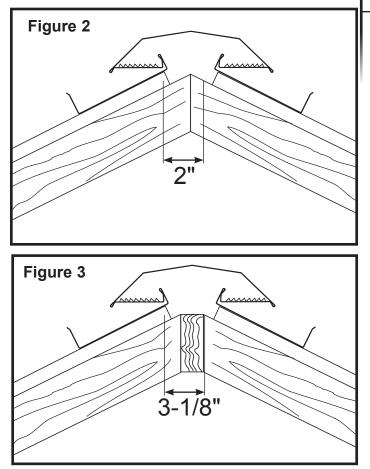
After determining the type of construction, mark the appropriate cut line. Be sure to begin and end the cut 6 inches inside the overall length of the vent as measured in Step 1 and Step 2.
