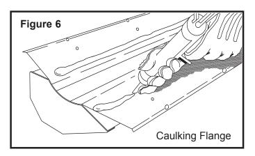
Align end of first section (with endplug installed) on the end marks and the bottom of the nailing flange on the chalk line. Then nail the section down using broad headed roofing nails, making sure to keep the bottom of the section aligned with the chalk line. As you proceed down the roof, caulk the male connection as shown in Fig. 7 and connect the male-female ends. Install the last end plug on the last vent section before nailing it down.
