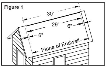
When you have determined the overall length of vent to be installed, center the measurement between the ends of the roof and mark these two points.
